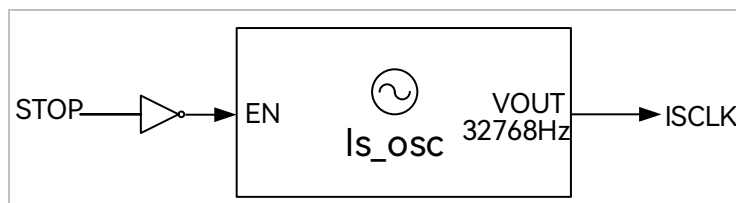
Figure 23-3 Input/Output of Internal Slow Clock on ISOSC Pin
